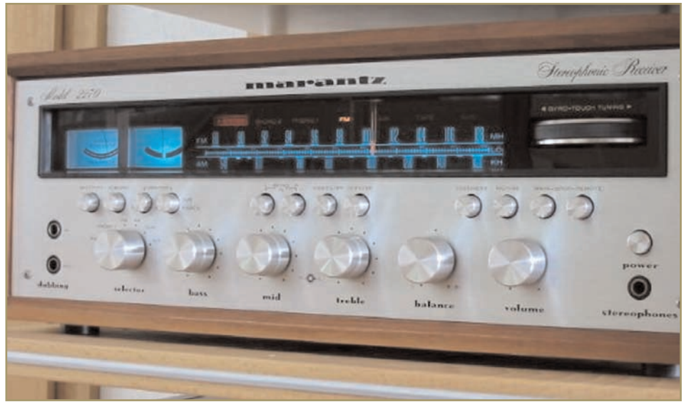
The Marantz 2270 Receiver. The model numbers of the “2200” series receivers included power ratings. In this case, power output was 70 watts per channel.
